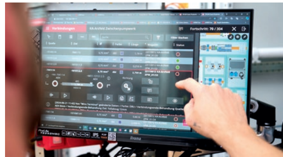
The Eplan Smart Wiring assistance system visualises the mounting layout, devices, connections and wiring routes and acts as a guide for the wiring process.
